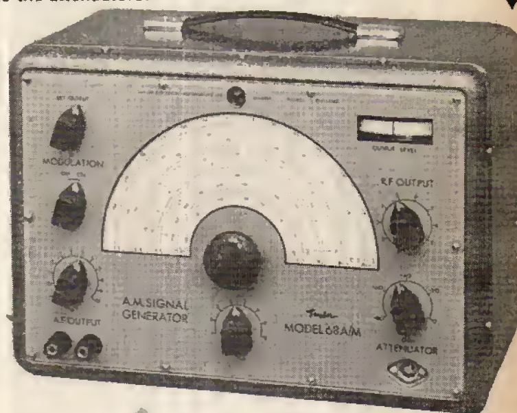
Fig. 16: The still popular Taylor Model 68A/M signal generator. Frequency range is from 100kHz to 240MHz (all on fundamentals) over 8 ranges. Although a.m. only, the instrument is suitable for the alignment of ratio detectors and f.m. r.f. and i.f. stages. A variable 400Hz audio output is available and an r.f. monitoring meter allows accurate setting of the signal applied to the attenuators.
